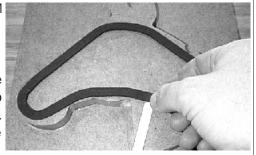
Woodworking:- Using Vac-Clamp with jigs
